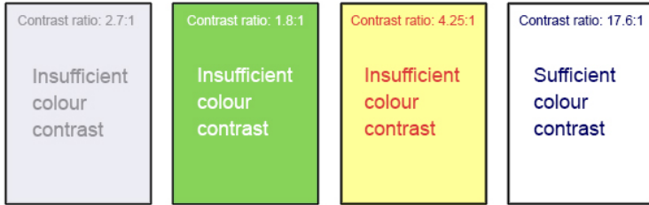
Image displays four examples of different font colour against different background colours; only one of the sample combinations provides sufficient colour contrast.
