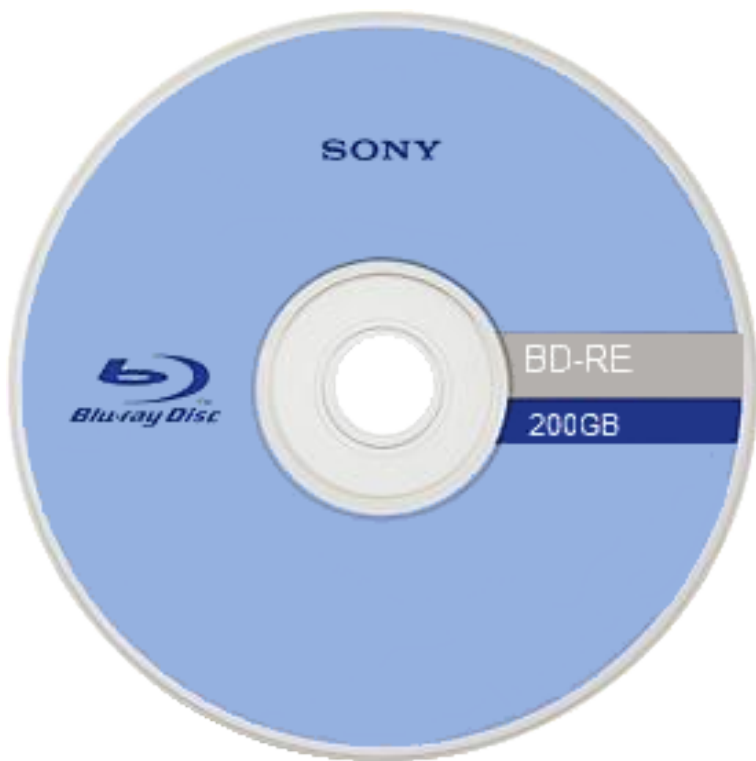
Figure 4.20: An Optical Disc (Blu-ray). Optical discs, such as CDs, DVDs, and Blu-ray discs, are a form of portable storage that are read by a laser. While less common for personal data storage today, they are still widely used for distributing software, movies, and video games. Image Credit: “Blu-ray 200GB” by Rtty66uyuyty is in the Public Domain, via Wikimedia Commons.
