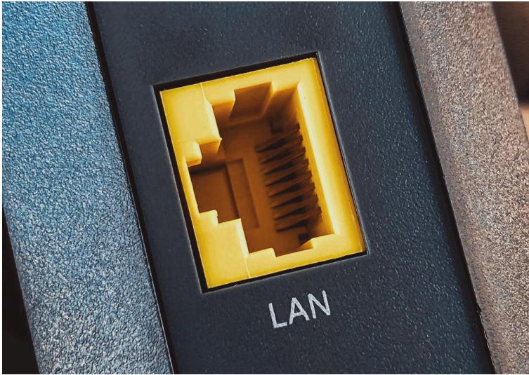
Figure 4.24: An Ethernet Port. An Ethernet port, also known as a LAN port, is used to connect a computer to a wired network using an Ethernet cable. While Wi-Fi is common, a wired connection often provides a faster and more stable internet connection, which is important for online gaming, streaming high-definition video, and transferring large files. Image Credit: “LAN Port – Ethernet Jack on Cable Modem (Networking Equipment)” by Tony Webster is licensed under CC BY 2.0, via Wikimedia Commons.
