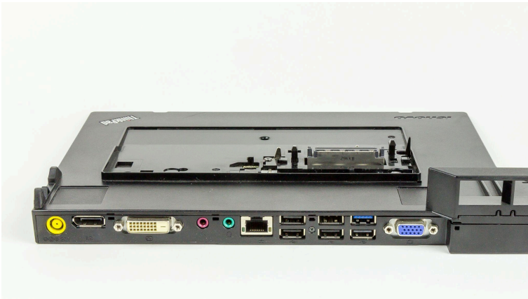
Figure 4.25: A Laptop Docking Station. A docking station is a device that allows a laptop computer to easily connect to other devices, such as a full-size monitor, keyboard, mouse, and a wired network. It turns a portable laptop into a more complete desktop setup, which is very common in modern business offices. Image Credit: “ThinkPad Mini Dock Series 3, Type 4337-9663” by Raimond Spekking is licensed under CC BY-SA 4.0, via Wikimedia Commons.
