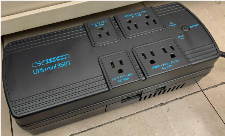
Figure 8.8: An Uninterruptible Power Supply (UPS). An essential device for critical systems like servers and important workstations. A UPS contains both surge protection circuits and a built-in battery. If there is a power failure, like a blackout, the battery instantly kicks in to provide power for a short time (usually 5-15 minutes). This isn't enough time to keep working for hours, but it gives you a crucial window to save all your files and shut down the computer properly, preventing any data loss. For a business server, this is absolutely essential equipment. Image Credit: “UPS_mini_350T” by Project Kei is licensed under CC BY-SA 4.0, via Wikimedia Commons.
