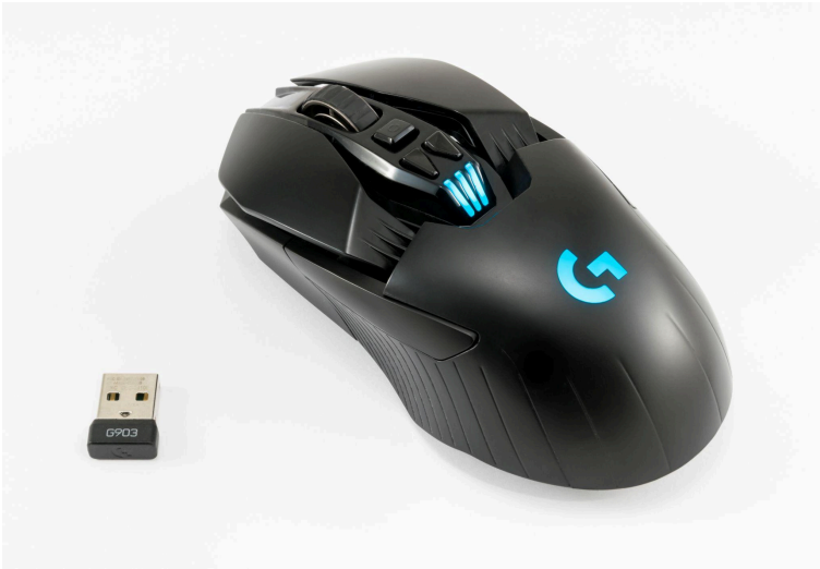
Figure 4.7: A Computer Mouse. The mouse is a pointing device that allows the user to move a cursor on the screen and interact with graphical elements. It is an essential input device for navigating the Graphical User Interface (GUI). Image Credit: “2023 Mysz komputerowa Logitech G903 Lightspeed” by Jacek Halicki is licensed under CC BY-SA 4.0, via Wikimedia Commons.
