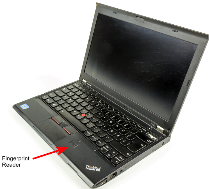
Figure 8.6: Biometric Authentication (Fingerprint Readers). An example of a laptop with a built-in fingerprint reader for biometric authentication. The tiny yellow arrow points to the small sensor on the palm rest, where a user would place their finger to log in instead of typing a password. Image Credit: “ThinkPad_X230-9671” by Raimond Spekking is licensed under CC BY-SA 4.0, via Wikimedia Commons.
