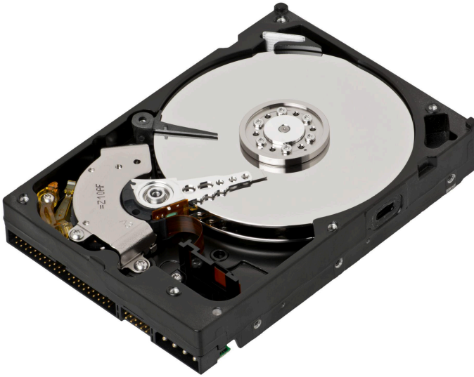
Figure 3.2: Hard Disk Drive (HDD). A Hard Disk Drive (HDD) is a primary example of a computer's permanent storage. It holds the operating system, all your installed programs, and personal files such as documents and photos. Unlike RAM, an HDD is non-volatile, meaning it retains all this information even when the computer is turned off. Image Credit: "Desktop Hard Drive" by George D. Darrin is licensed under CC BY-SA 4.0, via Wikimedia Commons.
