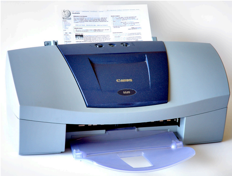
Figure 4.12: An Inkjet Printer. A printer is an output device that produces a physical copy, or 'hard copy,' of digital documents and images. Inkjet printers, like the one shown, are common for home and small office use and work by spraying tiny droplets of ink onto paper. Image Credit: "Canon S520 ink jet printer" by André Karwath aka Aka is licensed under CC BY-SA 2.5, via Wikimedia Commons.
