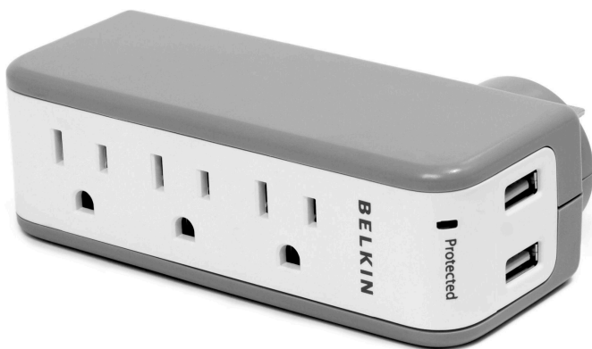
Figure 8.7: A surge protector. An example of a surge protector as an essential device that protects electronics from power spikes. While it may look like a normal power adapter or extension cord, it contains special electrical components that absorb the extra electricity during an overvoltage, sacrificing itself to save the connected equipment. The small light labeled “Protected” indicates that the safety feature is active. Every important piece of computer hardware, from a server to a desktop PC, should be plugged into a surge protector rather than directly into the wall outlet. Image Credit: “Belkin-Surge-Protector” by Evan-Amos is in the Public Domain, via Wikimedia Commons.
