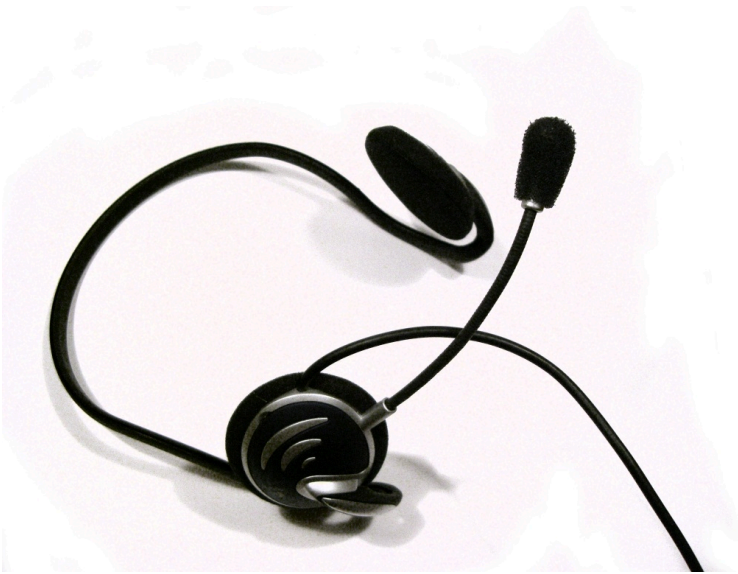
Figure 4.8: A Headset. A headset is a device that combines headphones (an output device for sound) and a microphone (an input device for sound) into a single unit. Headsets are commonly used for online meetings, gaming, and customer service calls. Image Credit: “Headphones with Microphone” by Zephyris is licensed under CC BY-SA 3.0, via Wikimedia Commons.
