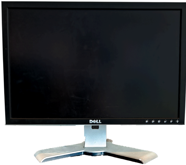
Figure 4.11: A Desktop Computer Monitor. The monitor is an output device that displays visual information from the computer. The quality of the image is determined by its resolution, which is the number of pixels used to create the image on the screen. Image Credit: “Dell Computer Monitor” by IT Photography is licensed under CC BY-SA 4.0, via Wikimedia Commons.
