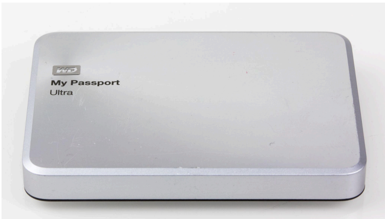
Figure 4.17: An External Hard Drive. An external hard drive is a portable storage device that connects to a computer, usually via a USB cable. It provides a convenient way to back up important files, store large amounts of data, and transfer files between different computers. Image Credit: “My Passport Ultra Metal Edition-2969” by Raimond Spekking is licensed under CC BY-SA 4.0, via Wikimedia Commons.
